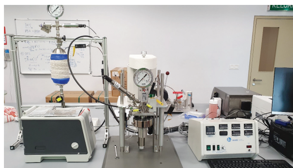
Fig.1 High Pressure CO 2 Absorption Setup
